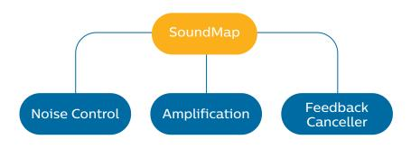
Figure 1: SoundMap covers the three pillars of sound processing in Philips HearLink: Noise Control, Amplification and Feedback Cancellation
