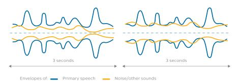
Figure 2: Envelopes of speech and noise at two different noise levels; low (left) and high (right)
