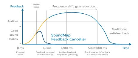
Figure 6: Growth and management of feedback in hearing aids. After an abrupt initial acoustical change around the hearing aid (e.g. phone to the ear), a feedback loop can be triggered, and feedback whistling may become audible. The figure shows the difference in reaction time between a traditional anti-feedback strategy, which often reacts after feedback has become audible and SoundMap Feedback Canceller, which can prevent feedback while it is still building up and not yet audible.
