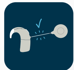
Antenna cable pull – 35 N (3.5 kg)
