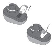
Open and close the battery drawer on the instrument(s), and place them close to your iPhone. The instrument(s) remains in pairing mode for 3 minutes
